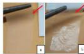
Figure 6. The film of solid biopolymer blend electrolyte representative (a) before and (b) after [EMIm]Ac ionic liquid incorporation.
